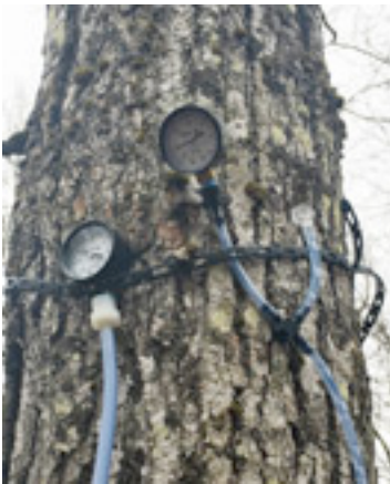
Figure 1. Maple tree with a 3/16" dropline and 5/16" dropline used to measure the difference achieved in vacuum from using 3/16" tubing, Paul Smith's College sugarbush, maple sap tubing systems evaluation, 2016.
