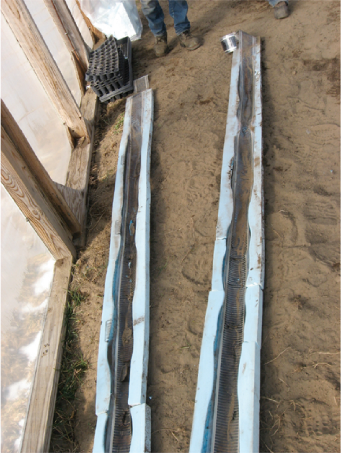
Photo 3. Melted 15 watt heat strips and insulation that were removed from two of the treatment beds on February 7, 2012. (Photo by Michael Davis)
