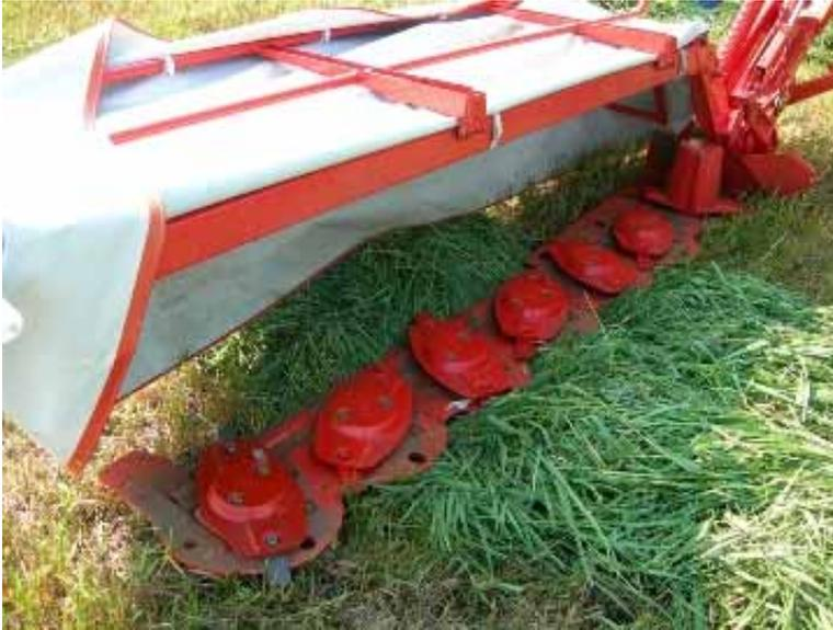
Kuhn mower without conditioner. This mower can produce a wide swath of approximately 90% by removing swath adjusters. Photo credit: D. Cherney.
