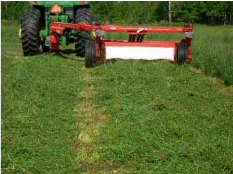
Kuhn mower-conditioner with wide swath attachment. A wide swath attachment allows an approximately 90% wide swath with conditioning. Photo credit: D. Cherney.
