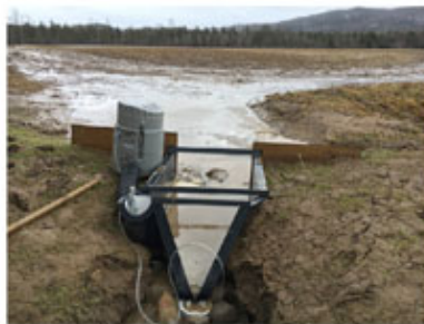
Figure 4, left: Flume capturing surface runoff during snowmelt event on 1/12/18 for undrained field, NNYADP Tile Drainage project, 2017.
